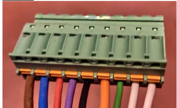
6 - Clip the new terminal onto the body with its 9-wire beam.
